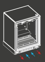
The air flows must not be mixed. Make sure that the incoming ai flow comes from outside by isolating the air flows. (By using adhesive foam for example)
